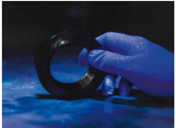
Test Fluid System for Penetration Testing
