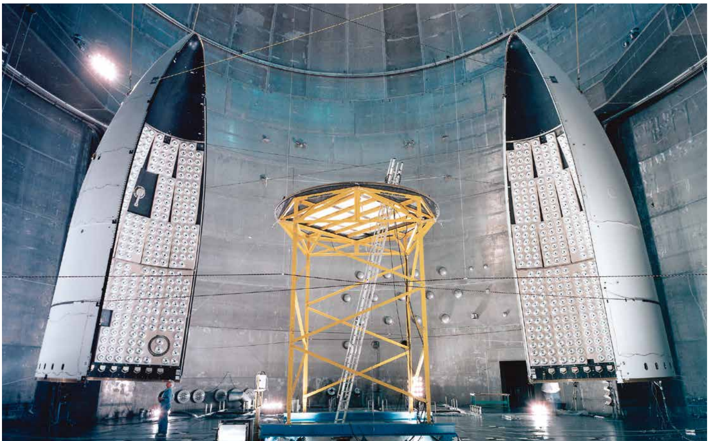
Payload Fairing Separation Test in the NASA Vacuum Chamber in Plum Brook Station, Ohio.
