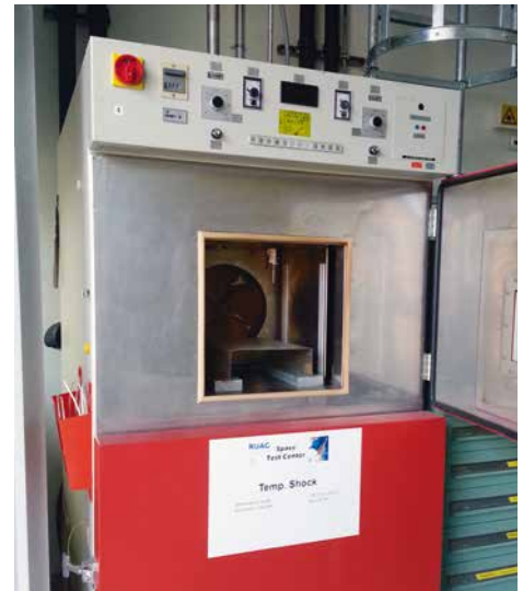
Temperature Shock Chamber
