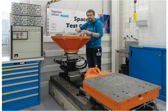
Shock Machine MTS
