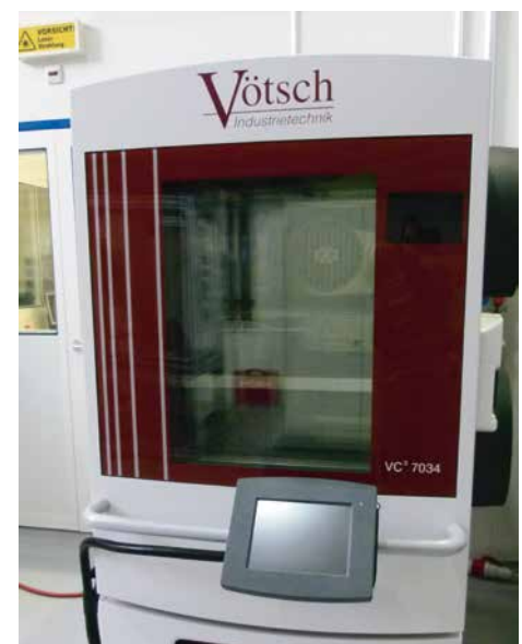
Vötsch VC 7034 Climatic Chamber
