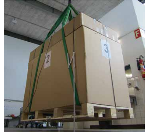
Drop Test of large objects
