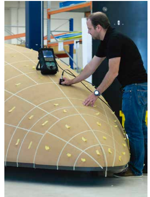
Ultrasonic NDI test on VEGA fairing
